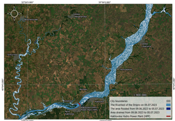
Difference in water mask for the upstream zone (geographical scope of water movement analysis) based on the satellite image from July 5, 2023
